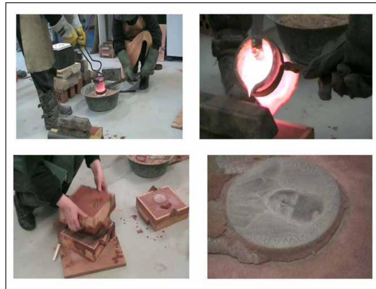
Fig 4. Sand casting demonstration
